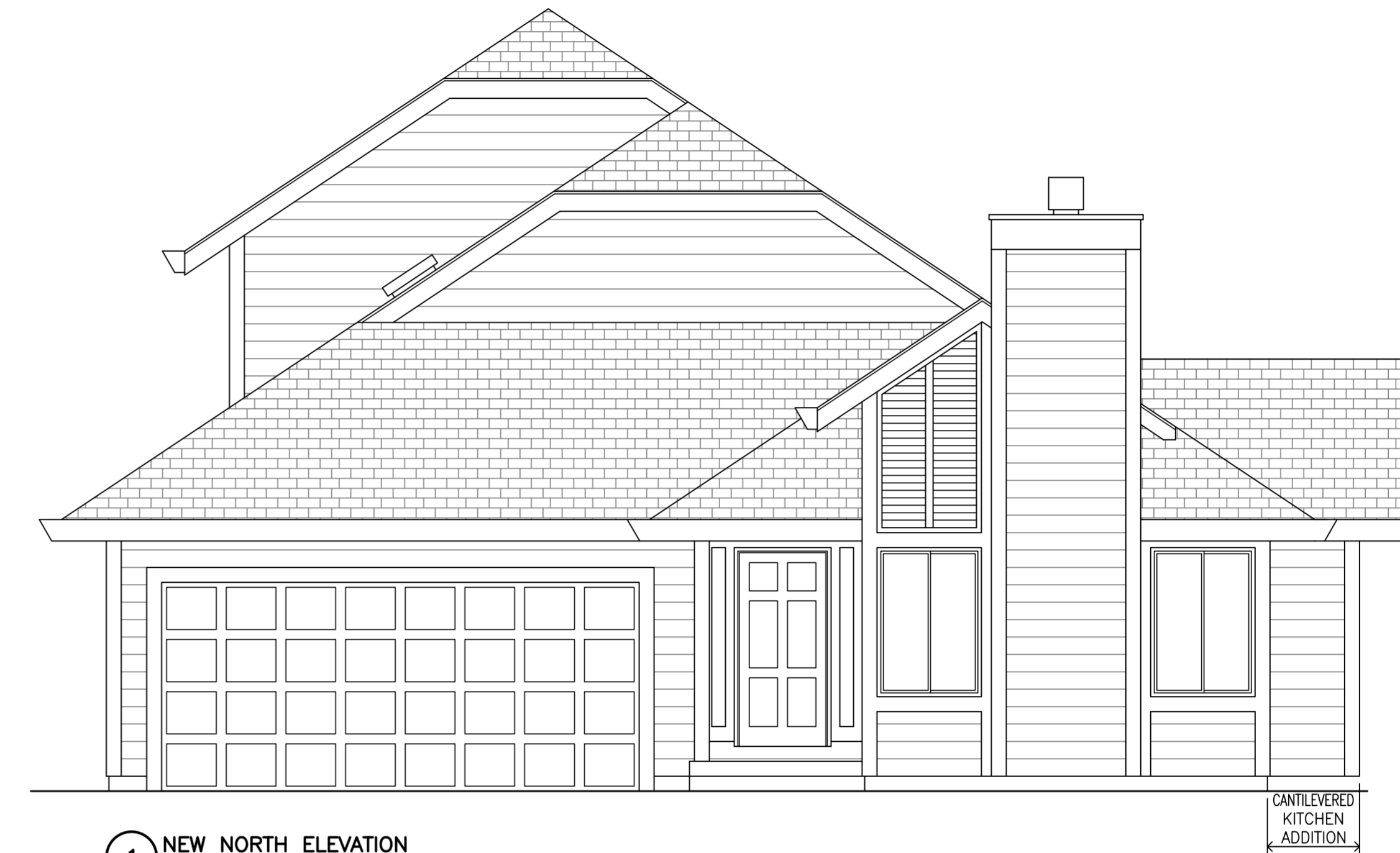
1 NEW NORTH ELEVATION 1/4" = 1'-0"
