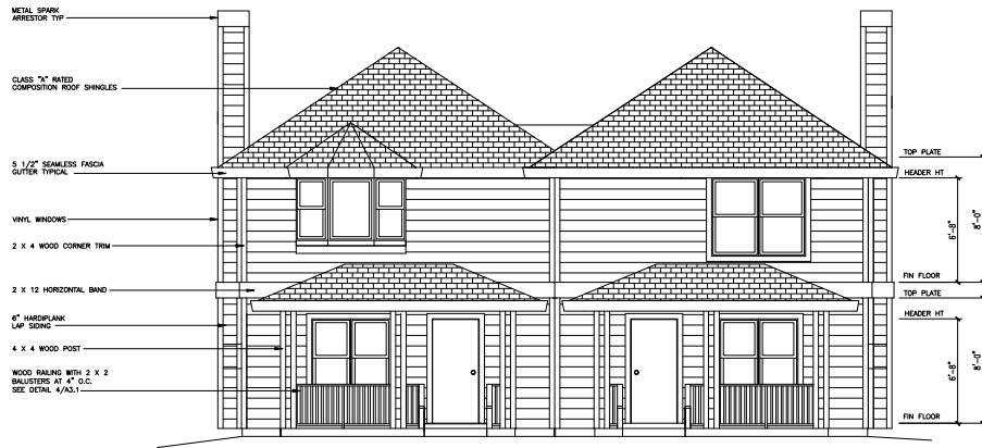
1 FRONT ELEVATION - BUILDING A 1/4" = 1'-0"
