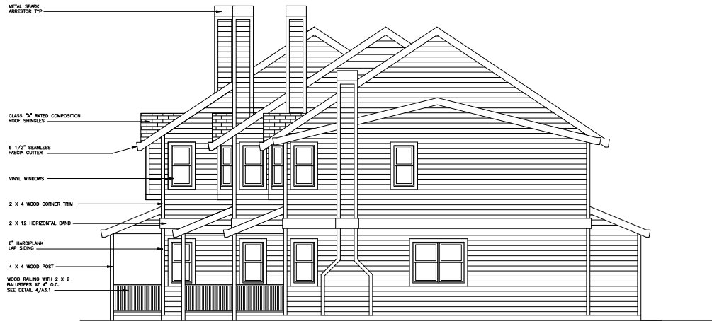
2 WEST ELEVATION - BUILDING B 1/8" = 1'-0"
