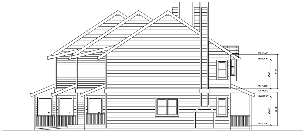
1 EAST ELEVATION - BUILDING B 1/8" = 1'-0"
