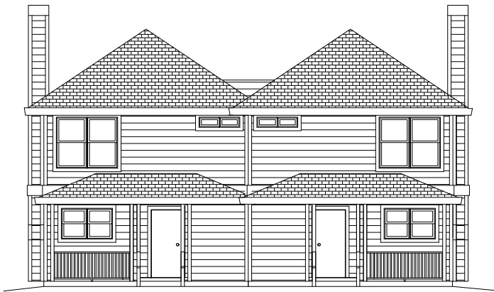
3 REAR ELEVATION - BUILDING A 1/4" = 1'-0"
